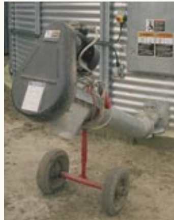
Grain is augered out of the bin by a 152mm horizontal and 200mm angled combination with 4kW motor
